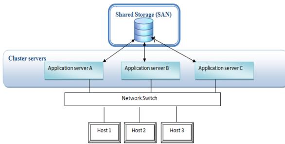
Fig. 2. Cluster Computing with SAN & Load Balancing
